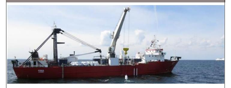
M/S Vina is a multipurpose DP1 Installation Vessel converted in 2010/14 and upgraded with a DP system 2014. It can operate worldwide, and can be adapted to many different tasks such as cable installation, survey & ROV-work and offshore diving.
